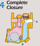
When condensate flow to the trap ceases, the float closes valve port (B) which is always sealed below the water level. The upper section fills with steam and the X-element closes valve port (A). The trap is then completely sealed, preventing any steam leakage.
